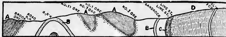
FIG. 11.— Geological Section of the Low Moor, Va., Iron-ore Bed. After B. S. Lyman, Trans. Amer. Inst. Min. Eng. , XIV., 801. A— Marcus Shale ; B— Oriskany Sandstone ; C— Lower Heblerberg Limestone ; D— Clinton Shales .
